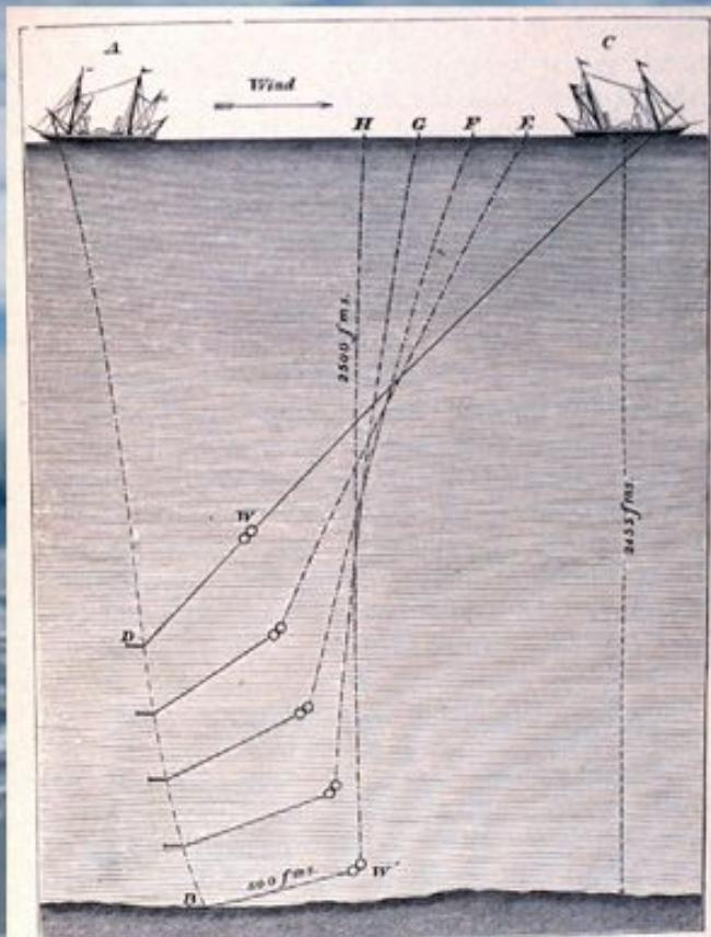
positions of the vessel, the weight attached 500
